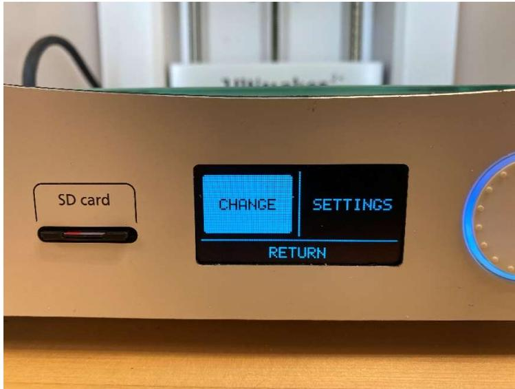
5.3.3 The machine will heat the filament, then back it out of the Canula.
