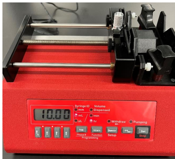
Figure 1: Syringe pump that is powered on with a number in the display panel and indicator lights for specified units of volume and time.
