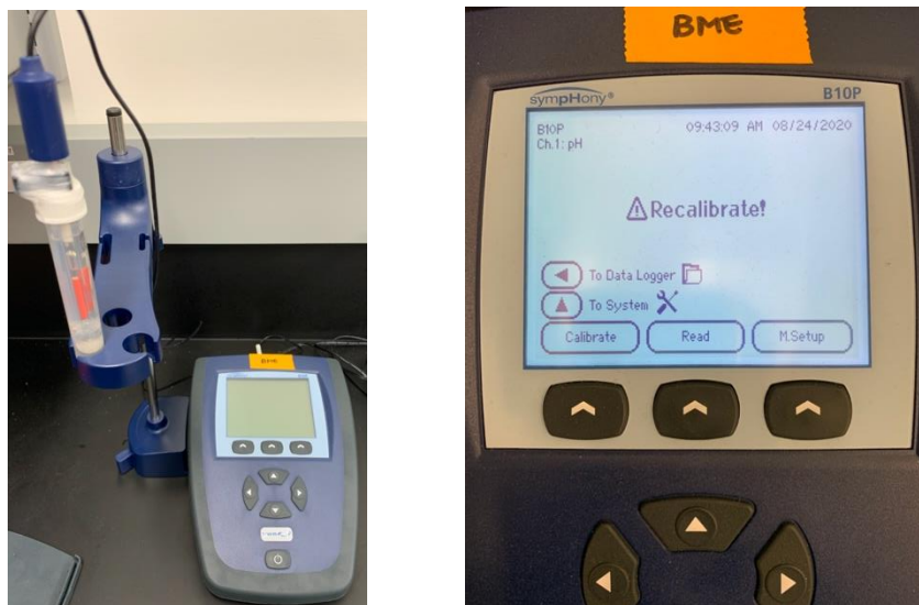
Figure 1. Left: the pH meter is composed of the main device and a pH probe that is immersed in storage solution. Right: the main screen after the instrument has been turned on.
