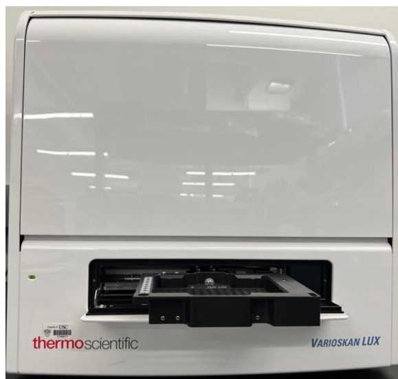
Figure 1: The plate reader with the plate slot open after initialization.
