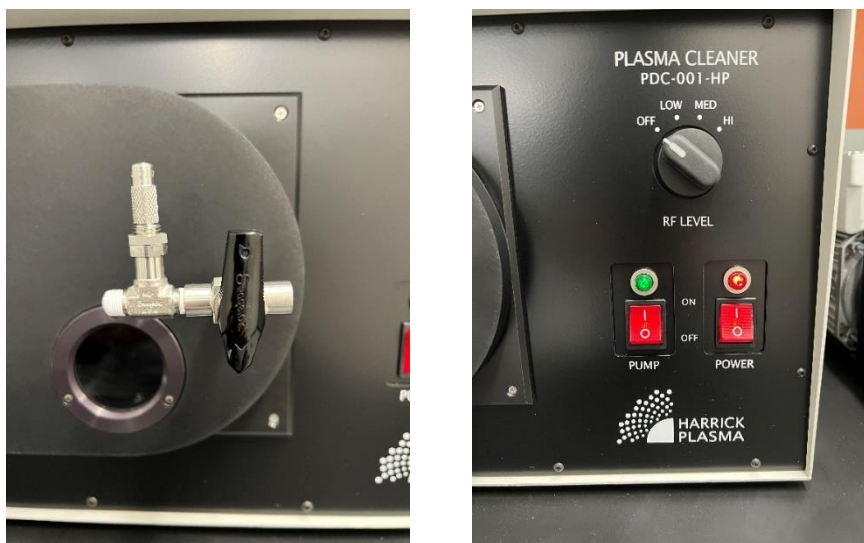
Figure 2: Left: The three-way valve in a closed configuration. Arrow denotes direction of the valve. Right: The set-up to initiate the plasma cleaner.
