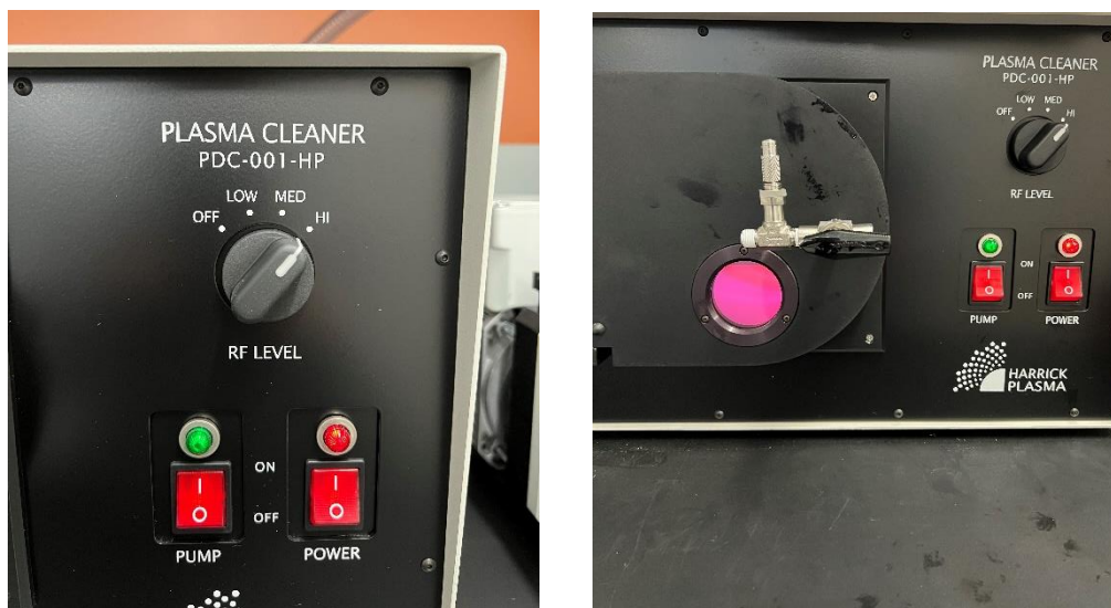
Figure 4. Left: The dial on the plasma cleaner to adjust the RF power level (low, medium, or high) – shown on “HI”. Right: The violet-pink glow in the chamber window when the RF level is selected.
