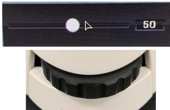
**Figure 6:** Slide bar on the monitor (top) or wheel on the bottom of the microscope (bottom) to adjust light intensity.
