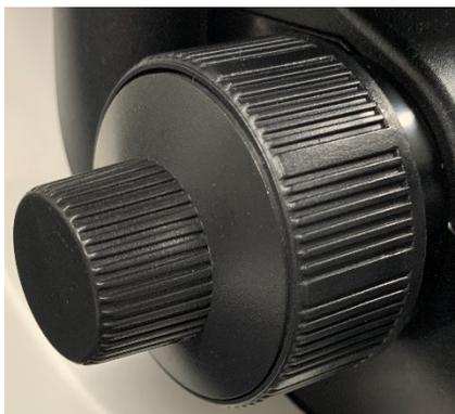
**Figure 5:** Focus knobs.
