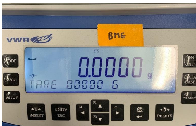
Figure 1. The main screen of the VWR-224AC analytical balance after zeroing the system.
