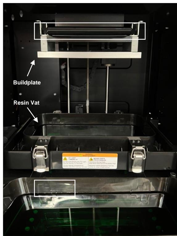
**Figure 2:** *Top:* Inside of the 3D printer with the buildplate and resin vat. White box indicates the “down” position. *Bottom:* Resin is filled close to the “bottom” step (white box).
