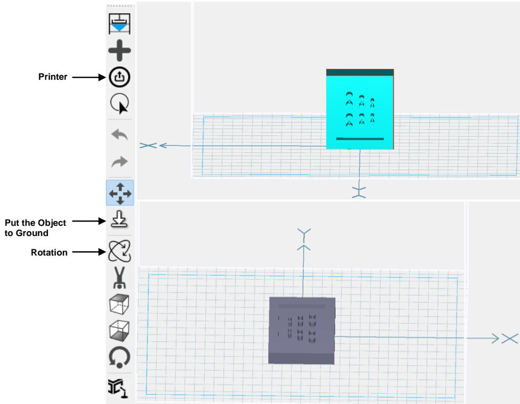
**Figure 3:** An example CAD file that needs to be rotated and positioned flat on the XY plane. The “Rotation” function rotates the design from a standing position to a flat configuration. The “Put the Object to the Ground” function positions the design directly on the XY plane. The “Printer” function converts the .stl file to a .slc file.
