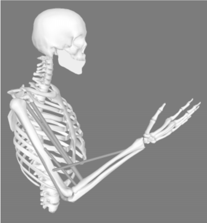
Figure 1 — Example arm model in SIMM window. SIMM uses such graphical user interfaces to accept user construction and modification of the modeled musculoskeletal components and to animate motion of the model system.
